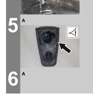
A Clean the seals between dirt water reservoir and cover and check for tightness, replace if required.
